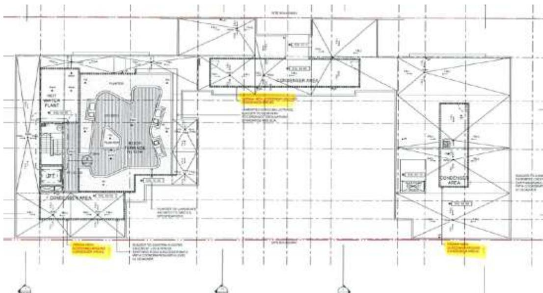
Figure 3. Roof plan showing x 3 locations of proposed plant screening (highlighted yellow). Note – Green Street to the right and Maroubra Road to the left.
